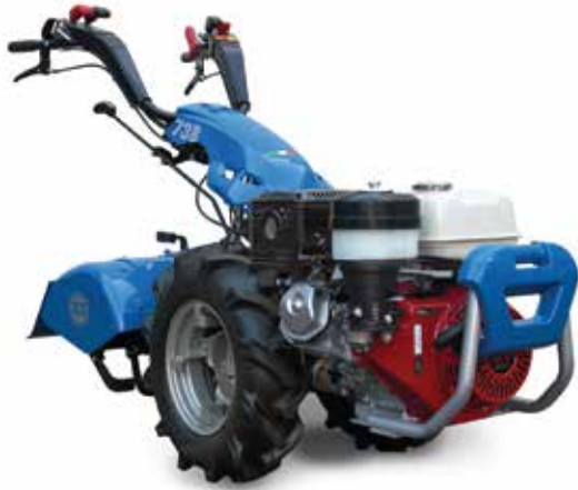
Two Wheel Tractor Powersave 738 Honda GX340E [recoil starter] Wheels 5.0-10 Without Rotary Hoe 8CCY65B0
